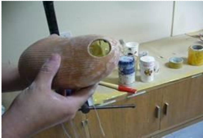
Fig.1 Seal the hold inside socket
